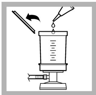
2. Open one m-FC broth ampule. Lift the cover of the filter assembly and pour the contents equally on the absorbent pad in the petri dish. Remove the petri dish from the filter assembly.
