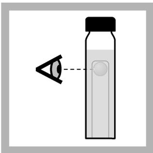
9. After  $24 \pm 2$  hours, remove the samples from the incubator. Gently tap each tube and examine the inner vials for gas. If the inner vial contains gas bubbles, the test is positive for fecal coliform bacteria. If none of the tubes contain gas, then the test is negative for fecal coliform bacteria.
