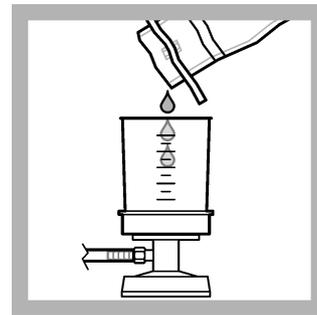
4. Pour 100 mL of the sample into the funnel. Pull the plunger on the syringe to pull the sample through the filter.
