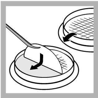
1. Use sterile forceps to put the membrane filter that is positive for total coliforms on the prepared NA/MUG agar plate. Let the membrane filter bend and fall equally across the agar to make sure that air bubbles are not caught below the filter.
