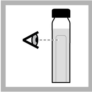
5. Examine the tubes to make sure that the inner vial (if Durham tubes are used) is full of liquid with no air bubbles.
