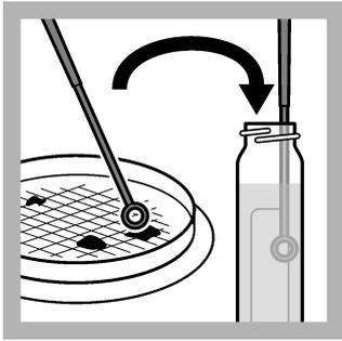
**1.** Use a sterile cotton swab or inoculating loop to touch all of the surface of the membrane filter that is positive for total coliforms.
