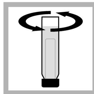
4. Invert the tubes to remove air from the inner vials. Gently swirl, if necessary.
