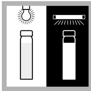
10. Apply UV light to the incubated sample that contains MUG broth with a long-wave UV lamp. Examine the tubes in a dark area. Look at the tube 90° from the UV light. Compare the fluorescence of the sample tubes to a tube that contains a known *E. coli* positive confirmation. If the sample fluoresces, *E. coli* bacteria are in the sample. If the sample does not fluoresce, the test is negative for *E. coli*.
