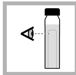
4. Examine the tubes to make sure that the inner vial (if Durham tubes are used) is full of liquid with no air bubbles.
