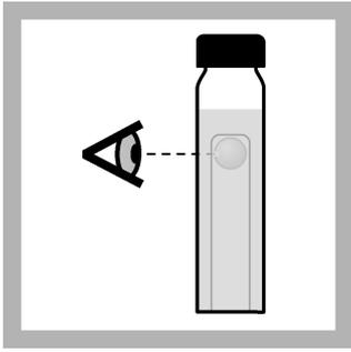
**9.** After  $48 \pm 3$  hours, gently tap each tube and examine the inner vials for gas. If the inner vial contains gas bubbles, the test is positive for total coliform bacteria. If none of the tubes contain gas, then the test is negative for total coliform bacteria.
