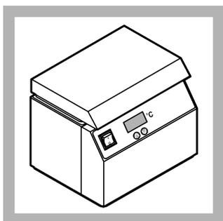
5. Incubate the inoculated confirmation media at  $35 \pm 0.5$  °C ( $95 \pm 0.9$  °F) for 1 hour. Bubbles that form in the inner vials during the first hour are not from bacteria.
