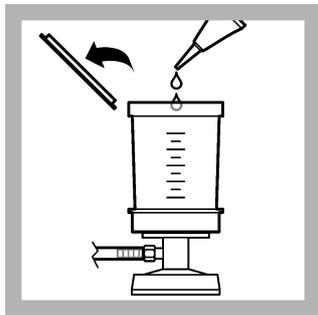
2. Open one m-Endo broth ampule. Lift the cover of the filter assembly and pour the contents equally on the absorbent pad in the petri dish. Remove the petri dish from the filter assembly.
