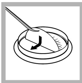
7. Put the membrane filter on the modified m-TEC prepared agar plate. Let the membrane filter bend and fall equally across the agar to make sure that air bubbles are not caught below the filter.
