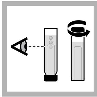
6. After 1 hour, invert the tubes to remove air from the inner vials. Make sure that there are no bubbles and keep the tubes in a vertical position. Loosen the caps only a little, then put the tubes in the incubator.
