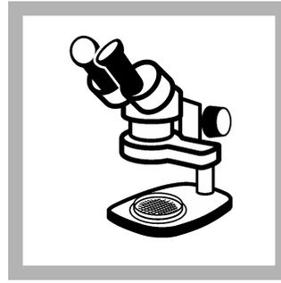
**11.** Remove the petri dish from the incubator. Use an illuminated magnifier or 10x to 15x microscope to count the number of colonies with a greenish-gold sheen. If the test is positive for coliform bacteria, start one or more confirmation procedures to confirm the presence of total coliforms, fecal coliforms or *E. coli*. Refer to [Interpret and report the coliform results](#) on page 9.
