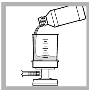
3. Pour 100 mL of the diluted sample into the funnel. Pull the plunger on the syringe to pull the sample through the filter.
