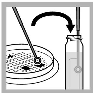
2. Swirl the cotton swab or inoculating loop in an EC/MUG Broth tube to move the colonies collected from the filter to the tube.
