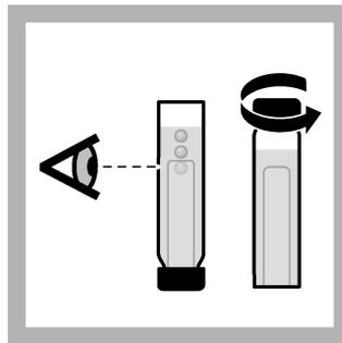
**7.** After 1 hour, invert the tubes to remove air from the inner vials. Make sure that there are no bubbles and keep the tubes in a vertical position. Loosen the caps only a little, then put the tubes in the incubator.
