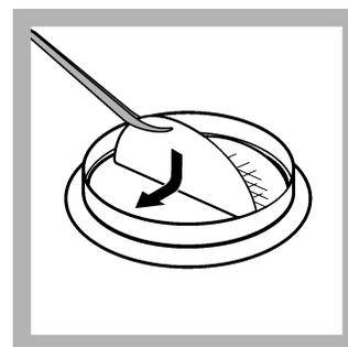
8. Put the membrane filter on the absorbent pad. Let the membrane filter bend and fall equally across the absorbent pad to make sure that air bubbles are not caught below the filter.
