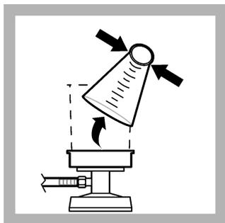
6. Squeeze the top of the funnel and remove the funnel from the filter assembly.
