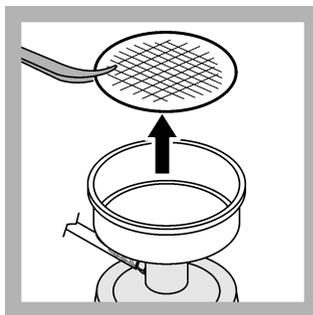
7. Use sterile forceps to lift the membrane filter from the base of the filter assembly.
