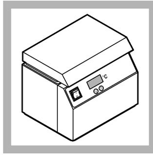
**10.** Incubate the inverted petri dish at  $35 \pm 0.5$  °C ( $95 \pm 0.9$  °F) for 22–24 hours.
