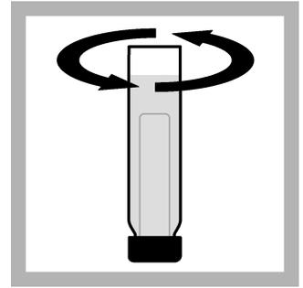
**4.** Invert the tubes to remove air from the inner vials. Gently swirl, if necessary.
