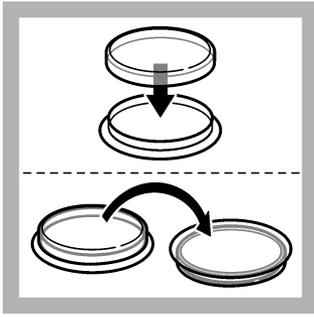
**9.** Put the lid on the petri dish and invert the petri dish.
