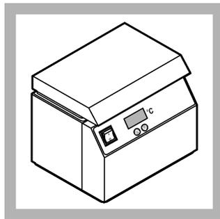
**6.** Incubate the inoculated confirmation media at  $44.5 \pm 0.2$  °C ( $112.1 \pm 0.4$  °F) for 1 hour. Bubbles that form in the inner vials during the first hour are not from bacteria.
