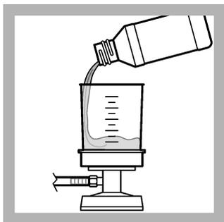
5. Rinse the funnel walls 3 times with 20 to 30 mL of sterile buffered dilution water. Use the syringe to pull the water through the filter after each rinse.
