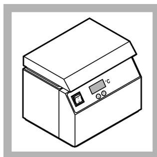
7. Incubate the inoculated confirmation media at  $35 \pm 0.5$  °C ( $95 \pm 0.9$  °F) for  $24 \pm 2$  hours. **Note:** It is necessary to keep the tubes in a vertical position for the remainder of the test.
