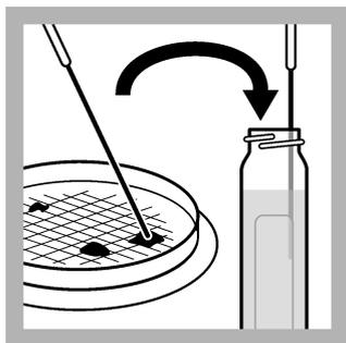
2. Touch the sterilized inoculating needle again to the same coliform (sheen) colony growth. Put the needle in a Brilliant Green Bile (BGB) broth tube.
