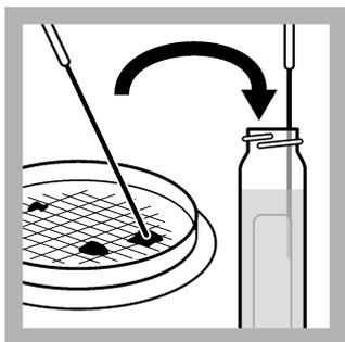
1. Touch a sterilized inoculating needle or a sterile disposable needle to the coliform (sheen) colony growth. Put the needle in a Lauryl Tryptose broth tube.
