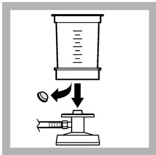
1. Remove the plug from the filter assembly. Push the filter assembly on the manifold.
