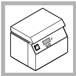
**13.** Incubate the inoculated confirmation media at  $44.5 \pm 0.2 \text{ }^{\circ}\text{C}$  ( $112.1 \pm 0.4 \text{ }^{\circ}\text{F}$ ) for 1 hour. Bubbles that form in the inner vials during the first hour are not from bacteria.
