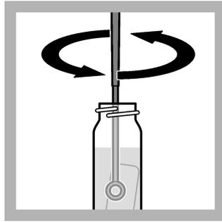
**2.** Swirl the cotton swab or inoculating loop in an EC Medium Broth tube to move the colonies collected from the filter to the tube.
