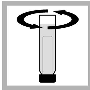
11. Invert the tubes to remove air from the inner vials. Gently swirl, if necessary.
