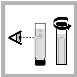
**14.** After 1 hour, invert the tubes to remove air from the inner vials. Make sure that there are no bubbles and keep the tubes in a vertical position. Loosen the caps only a little, then put the tubes in the incubator.
