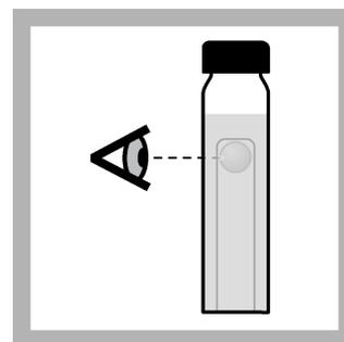
8. After  $24 \pm 2$  hours, remove the samples from the incubator. Tap each tube gently and examine the inner vials for gas. If the broth is cloudy and the inner vials contain gas bubbles, coliform bacteria are likely in the sample. Any gas that shows is an indication of coliform bacteria. If no gas can be seen, put the tubes in the incubator for  $24 \pm 2$  hours ( $48 \pm 3$  hours total) and examine the tubes again.
